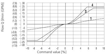
$Q_n = 15 \text{ II/min (4.0 GPM) by } \Delta p = 10 \text{ bar (145 PSI)}$
