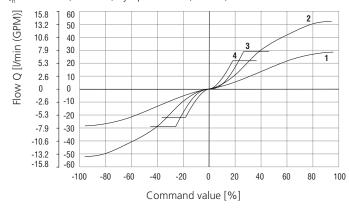
ninus load pressure  $\Delta p_n = 10 \text{ bar } (145 \text{ PSI})$   $\Delta p = 160 \text{ bar } (2321 \text{ PSI})$   $\Delta p = 50 \text{ bar } (725 \text{ PSI})$   $\Delta p = 320 \text{ bar } (4641 \text{ PSI})$
