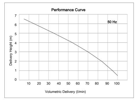
Kinematic viscosity : 90 mm²/s Operating temperature : 0.....60 °C
